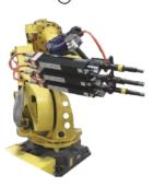
Multi Spindle Robot end effector solution with advanced tightening strategies, error proofing and data collection, reconfigurable for optimum productivity
