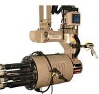
Custom 10 Spindle wheel multiple solution with advanced tightening strategies, error proofing and data collection for optimum quality
